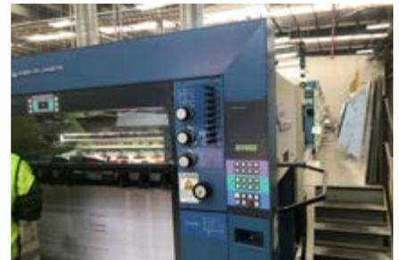
Our multi-colour offset printing presses can apply speciality finishing, such as UV varnish, in-line with a printed sheet size up to 1020 x 1420mm.
