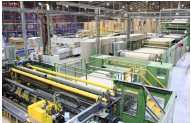
ABBE makes all of its own corrugated cardboard in many different specifications and paper grades. Our flute profiles include B, C, E, BC and EB. We can produce a sheet up to 2480 x 5000mm long.
