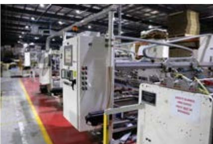
Our large format Gluing machines are capable of gluing large items like dump bins and display bases in a single piece.
